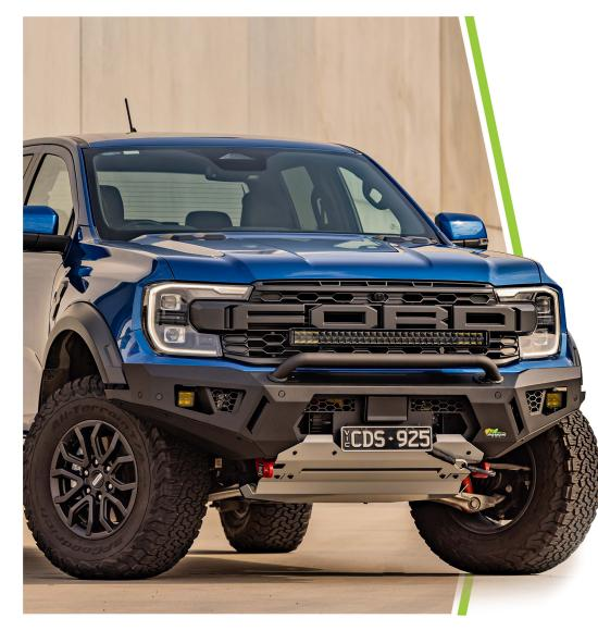
\*Fitting a lightbar to the centre hoop may impede some vision in the forward facing camera.
